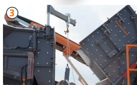
Blow-bar exchange system
