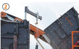
Blow-bar exchange system
